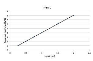
(c) Hang the mass from the string and attach the top of the string to a fixed point. Pull the mass back a small angular displacement (~ 10 degrees) and release. Use a stopwatch to time 20 oscillations, and divide the total time by 20 to obtain the period.
